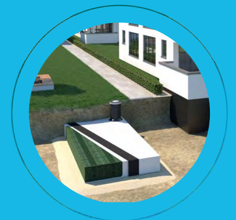
REGENWASSERSPEICHER (Rigolen Systemkonfiguration, Installation)
